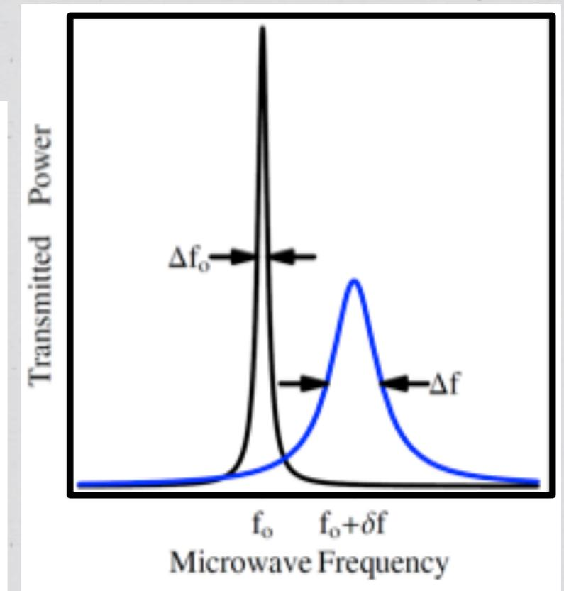
\* Cavity perturbation : a precise determination of  $\Delta\lambda$ .
