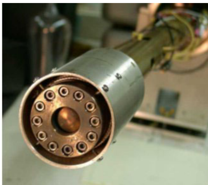
Muon's-eye view of the target cell, which is made of titanium and can withstand pressures of 500 bar at temperatures up to 500 °C. The dome shaped window is over 2 mm thick.
