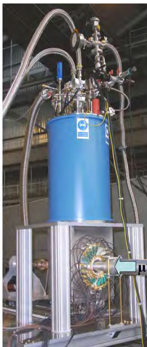
Left: 9.5 T magnet with detector system installed at PSI. Right: First data obtained at 9.5 T transverse field on a silver plate. Red curves represent the results from a fit in the time domain (time window 10 \mu s) and its Fourier transform.
