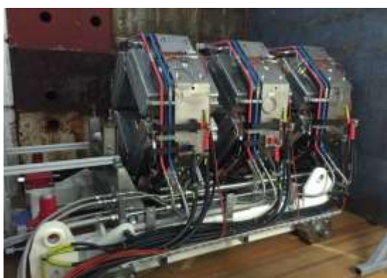
Fig ISIS1: The new quadrupoles (radiation hard) closest to our target shortly before installation. These magnets were made in house.
