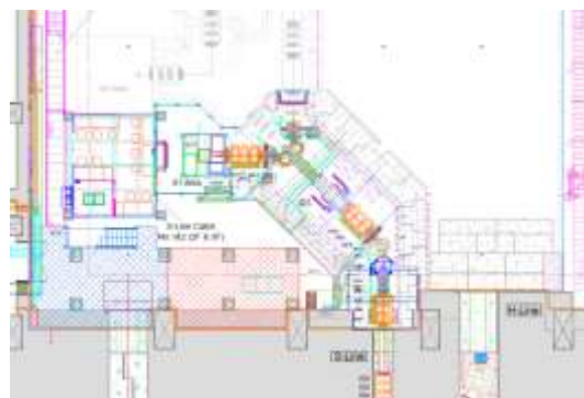
Fig. 2: Beamline layout of the S-Line (phase1).
